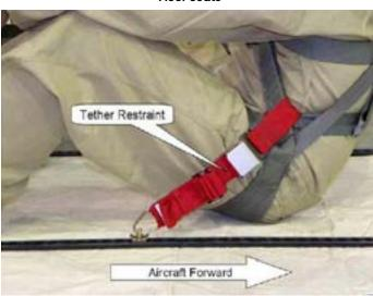
Figure 5. Pass Tether Loop Under Main Lift Web
