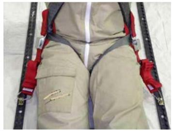
Figure 6. Latch Tetcher Loop Around Parachute Harness
